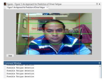
**Figure 5:** Fatigue Detection process initiated when the eyes of the person are open and the eye area are sliced means it shows the possibale Fatigue Detection.
